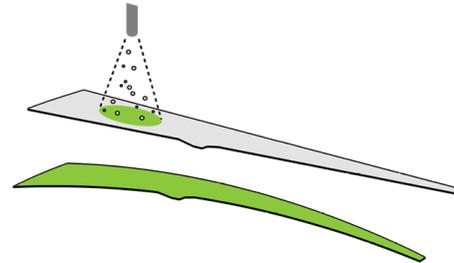
This project aims to develop a fully automated peen forming system based on numerical models and quasi-real time 3D shape measurements. We will demonstrate the possibility of automating the process and maximizing its robustness by incorporating modeling and 3D shape measurement in the control loop for on-line calibration and adaptive adjustment of the model with the feedback from shape measurement during peen forming.
